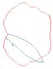
EWNA Type III - Asymmetric Wide (A3) 4,090 Lumens, 5000K (EWNA_A3550__-120-277V.IES)
