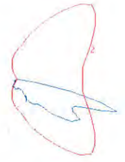
EWNA Type IV - Asymmetric Forward (A4) 3,750 Lumens, 5000K (EWNA_A4550__-120-277V.IES)
