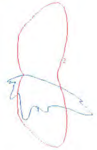
EWNA Type II - Asymmetric Narrow (A2) 3,960 Lumens, 5000K (EWNA_A2550__-120-277V.IES)
