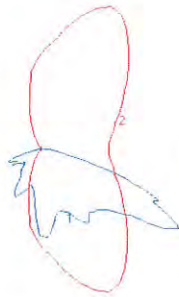
EWNA Type II - Asymmetric Narrow (F2) 13,080 Lumens, 5000K (EWNA_F2550__.IES)
